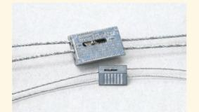
KwikWire system is designed to provide an economical alternative to jack chain and threaded rod when supporting wire basket and other cable support systems. Simple height adjustments are made by releasing locking tab, no tools required. Wire can be field cut to size, reducing waist and up front planning. KwikPak includes supply of clamps and spool of wire.
